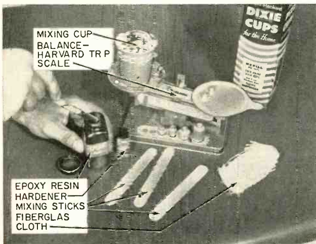
Fig. 2 —Equipment and materials for mixing the resin.
